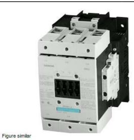
CONTACTOR, 75KW/400V/AC-3, AC(40...60HZ)/DC OPERATION UC 23...26V AUXIL. CONTACTS 2NO+2NC 3-POLE, SIZE S6 WITH BOX TERMINAL
